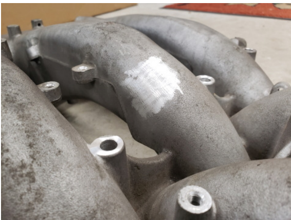
Figure 4 – Early and Late #3 runner boss removed
