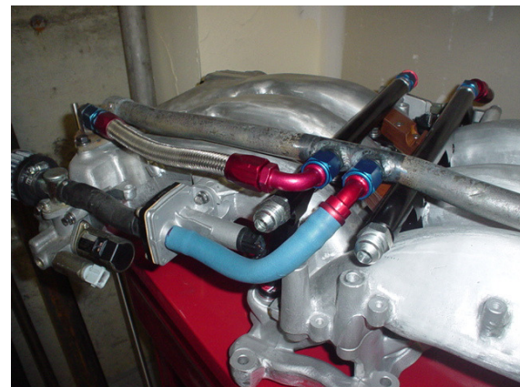
Figure 7 – Idle air plumbed with AN hose fittings
