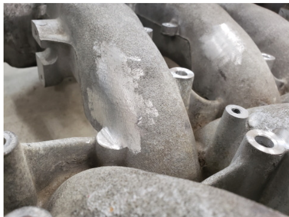
Figure 5 – Late #5 runner mod for #6 inj clearance
