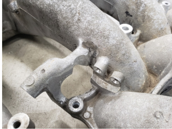
Figure 3 – Late mod for #1 injector clearance
