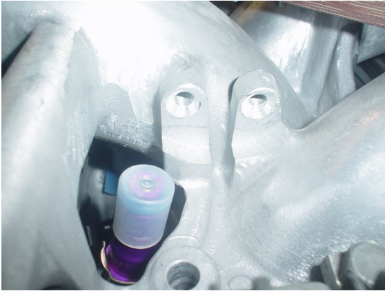
Figure 8 – countersunk bolt holes
